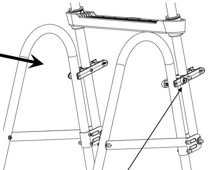
The Swivel Ladder Clamp with Button will automatically latch to the Ladder Handle in the upright position when idle. Press the button to unlock the ladder.
